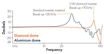
The frequency at which the dome begins to break up (distortion) is proportional to  $\sqrt{(E/\rho)}$  where E is Young's Modulus and  $\rho$  is density. As shown in the graph, synthetic diamond domes, in this instance having radius of curvature of 20 mm, offer the best FoM against competing solutions. Their geometry can be tailored to specific applications, delivering the best possible performance at every listening experience.
