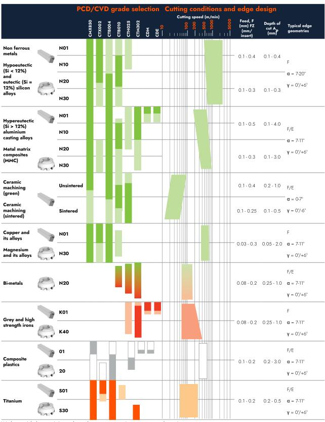
Work material characteristics and, to a lesser extent, cutting parameters, determine the demands placed on the cutting tool and, hence, the optimum balance of tool material properties. Knowledge of the application, including workpiece composition, facilitates selection of the optimum grade and correct tool geometry. Often, work material composition and machining parameters (vc, f, ap) are closely correlated. It is possible, therefore, only to provide a typical range of values for each parameter.
