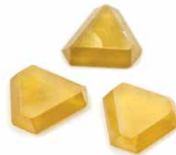
High pressure high temperature synthetic diamond is usually nitrogen doped, giving it a distinctive yellow hue.
