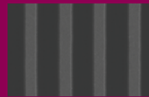
Figure 4: Trenches of equal periodicity and depth created by innovative etching technology to produce QWP
