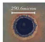
Laser induced damage of AR coating.
