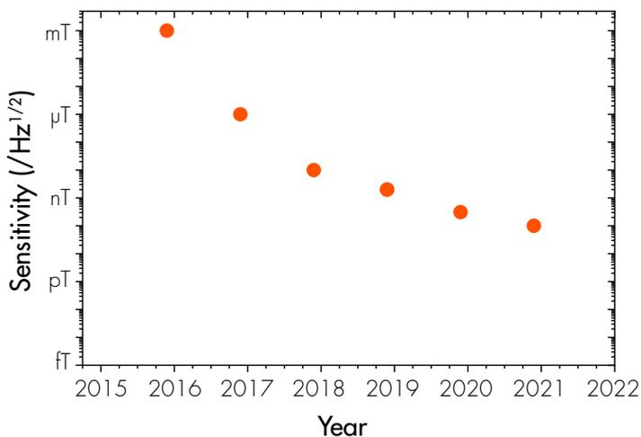
The fibre-coupled diamond magnetometer at the University of Warwick has been improved in sensitivity by a factor of 10 million in five years.
